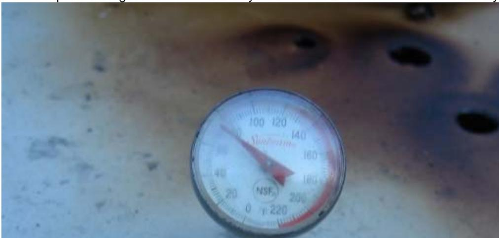
Here are the thermometers that are on the outside so I can see the temperature inside. I just bought oven thermometers that go fro 100 to 400 degrees and drilled a hole to put them in.
