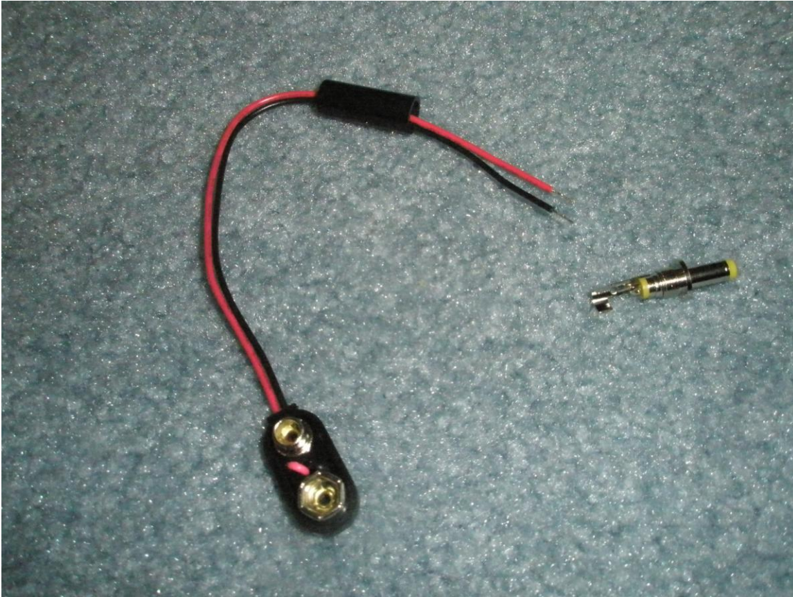
Photo #2 showing power plug disassembled and leads routed through backshell
