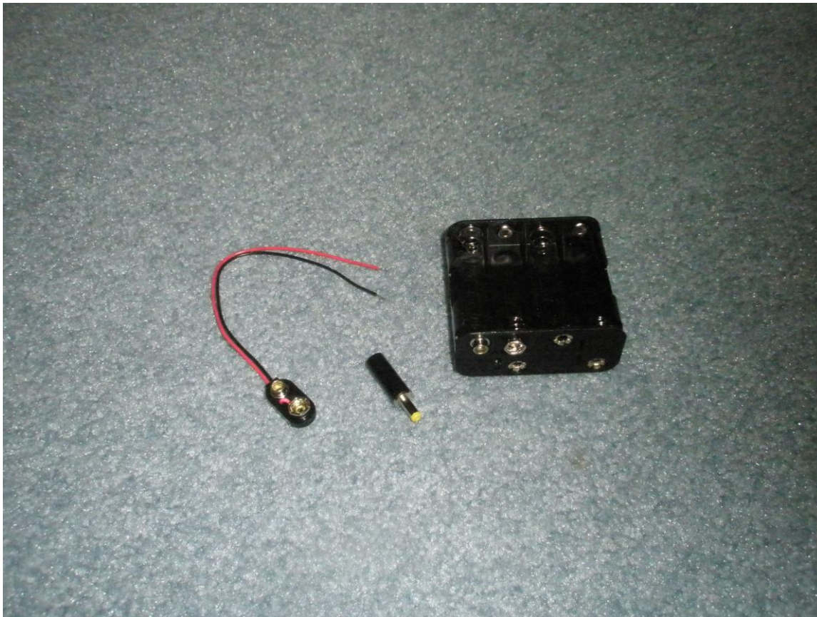
Photo #1 showing (from left to right) snap connector (270-0324), power plug (274-1532), and battery case (270-387).
